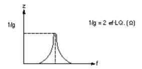
When Rd is connected to the hysteresis pin,  $(Rd + r_{cs} // Rh)$  1/g is the condition for oscillation to start, and (Rd + Rh) > 1/g is the condition for oscillation to stop. Note that  $r_{cs}$  is the internal resistance of the hysteresis pin.
