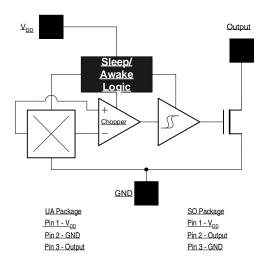
**Note:** Static sensitive device; please observe ESD precautions. Reverse V<sub>DD</sub> protection is not included. For reverse voltage protection, a 100W resistor in series with V<sub>DD</sub> is recommended.
