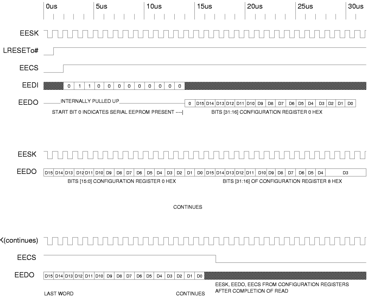
Timing Diagram 2-1. Initialization from Serial EEPROM (2K Bit)
