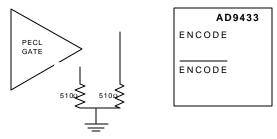
Figure TBD. Using PECL to drive the ENCODE Inputs
