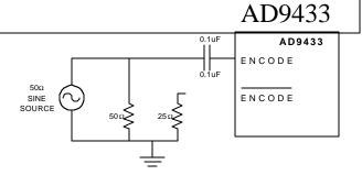
Figure TBD. Single ended 50 Sine Source Encode Circuit **ENCODE Voltage Level Definition**
