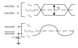
Figure TBD. Differential and Single Ended Input Levels **Analog Input**
