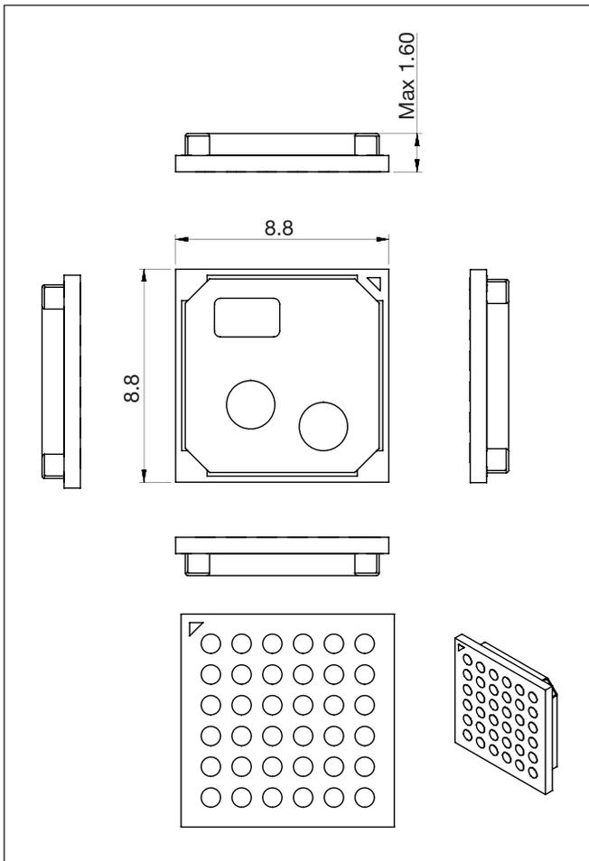
Figure 3. Mechanical dimensions and footprint.
