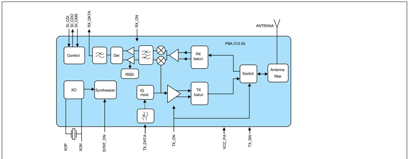
Figure 4. PBA 313 05 block diagram
