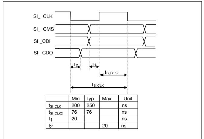
Figure 7. Timing diagram of the serial interface.
