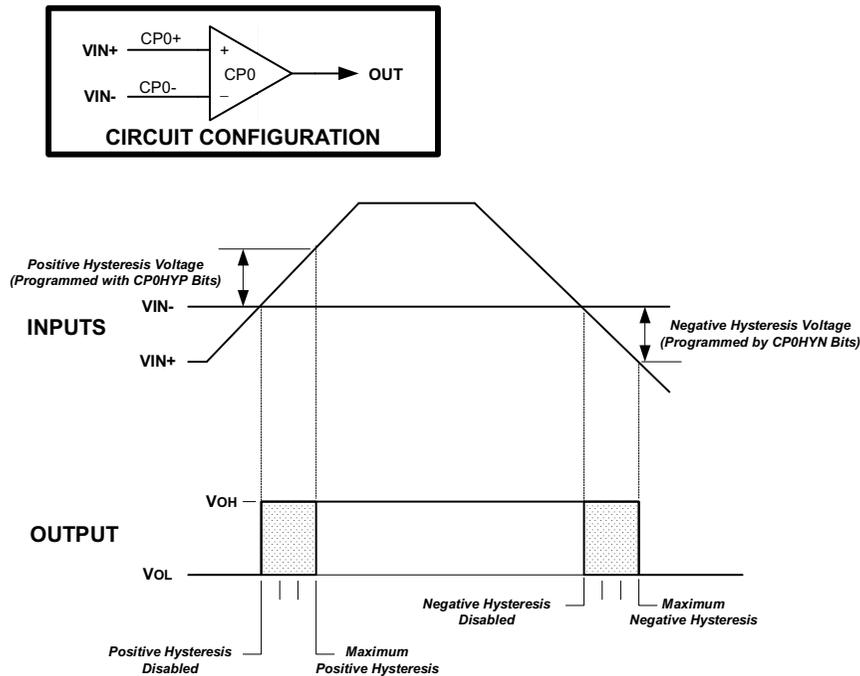
The Comparator hysteresis is software-programmable via its Comparator Control register CPTnCN (for  $n = 0$  or  $1$ ). The user can program both the amount of hysteresis voltage (referred to the input voltage) and the positive and negative-going symmetry of this hysteresis around the threshold voltage.
