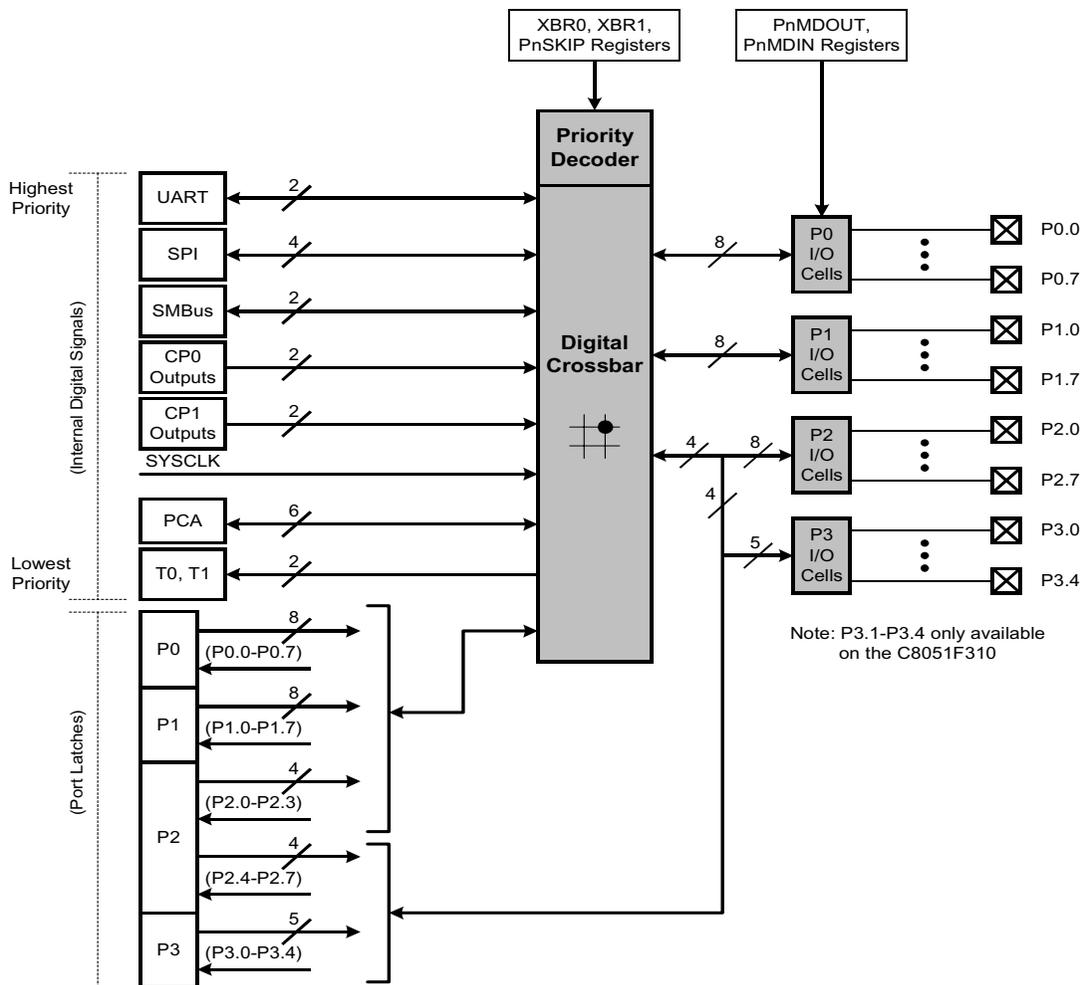
Figure 13.2. Port I/O Cell Block Diagram
