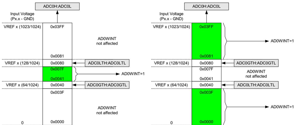
**Figure 5.17. ADC Window Compare Example: Left-Justified Single-Ended Data**
