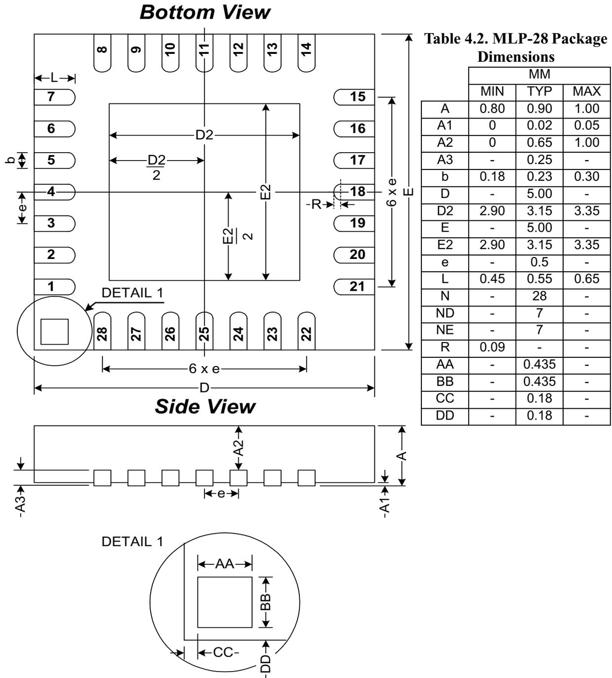
Figure 4.5. Typical MLP-28 Landing Diagram
