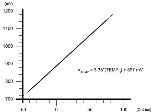
The uncalibrated temperature sensor output is extremely linear and suitable for relative temperature measurements (see Table 5.1 for linearity specifications). For absolute temperature measurements, gain and/or offset calibration is recommended. Typically a 1-point calibration includes the following steps:
