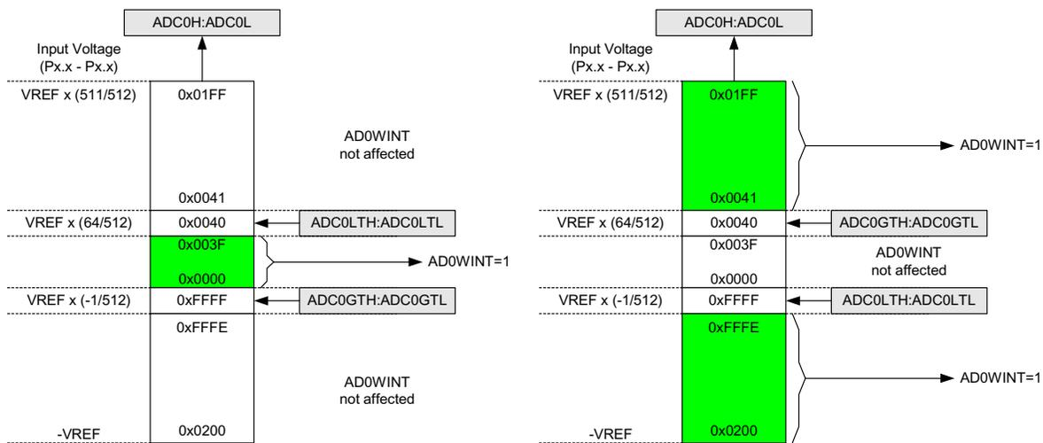
Figure 5.19. ADC Window Compare Example: Left-Justified Differential Data
