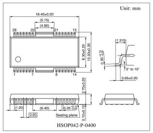
Note) The package of this product will be changed to lead-free type (HSOP042-P-0400D). See the new package dimensions section later of this datasheet.
