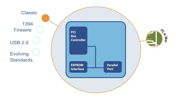
The Oxford PCI840 integrates a comprehensive parallel port and bridge to PCI.
