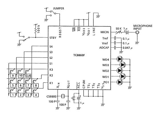
Note: External capacitors and resistors should be arranged as near TC8860F as possible.
