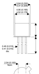
ტ 3 Bipolar NPN Device in a Hermetically sealed TO18 Metal Package.
