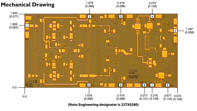
Units: millimeters (inches) Bond pad dimensions are shown to center of bond pad. Thickness: 0.110 +/- 0.013 (0.0043 +/- 0.0004), Backside is ground, Bond Pad/Backside Metallization: Gold All DC/IF Bond Pads are 0.100 x 0.100 (0.004 x 0.004). All RF Bond Pads are 0.100 x 0.200 (0.004 x 0.008) Bond pad centers are approximately 0.109 (0.004) from the edge of the chip. Dicing tolerance: +/- 0.005 (+/- 0.0002). Approximate weight: 4.787 mg.
