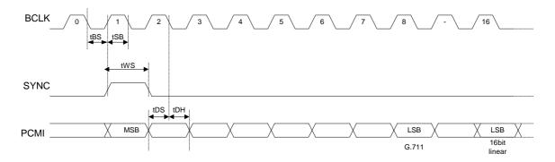
Fig. 2 PCM I/F mode input timing (long frame)
