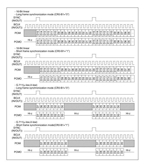
Fig. 11 PCM I/F mode timing diagram
