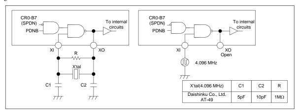
Fig. 10 Examples of oscillator circuit and clock input
