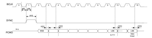
Fig. 5 PCM I/F mode output timing (short frame)
