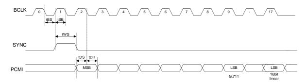
Fig. 3 PCM I/F mode input timing (short frame)
