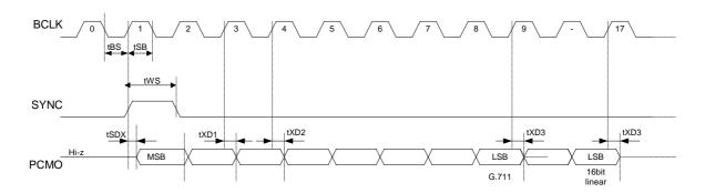
Fig. 4 PCM I/F mode output timing (long frame)
