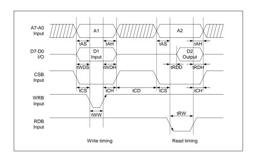
Fig. 6 Control register interface
