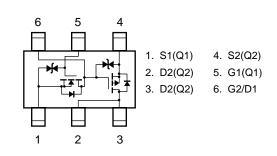
Remark The diode connected between the gate and source of the transistor serves as a protector against ESD. When this device actually used, an additional protection circuit is externally required if a voltage exceeding the rated voltage may be applied to this device.
