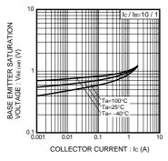
Fig.7 Base-Emitter Saturation Voltage vs. Collecter Current
