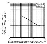
Fig.10 Collector Output Capacitance : Cob
