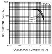
Fig.4 DC Current Gain vs. Collector Current (II)
