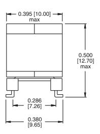
$\label{eq:Dimensions} \begin{tabular}{ll} Dimensions are in inches [millimeters]. \\ Standard dimension tolerance is $\pm 0.005 \ [0.13]$ unless otherwise noted. \\ \end{tabular}$
