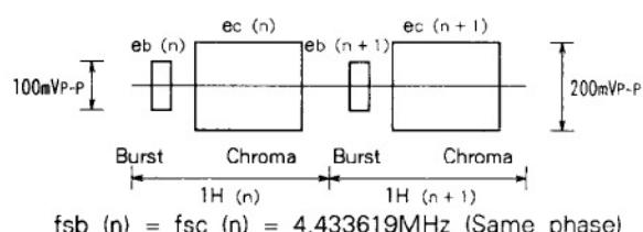
The phase relation of the above signal is as shown on the right. The phase relation of ec(n) and ec(n+1) to the burst may not always be as shown in the figure above: the test items for the phase relation in particular should be variable.
