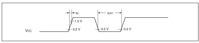
Note: Sudden change of power supply voltage may activate the power-on reset function. When changing power supply voltages during operation, set the slope of rising within 20 mV/ms as shown below.
