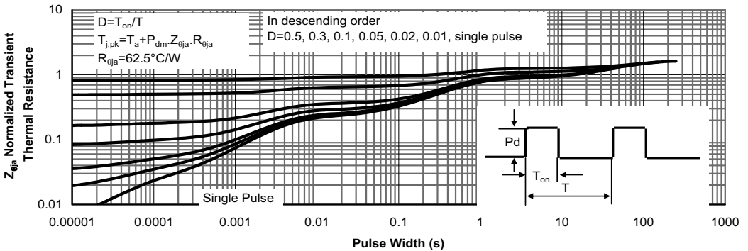
Figure 11: Normalized Maximum Transient Thermal Impedance
