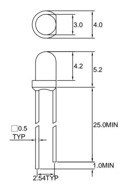
NOTE:1.All dimension are In millimeters tolerance Is  $\pm 0.25$  unless otherwise noted 2.Specifications are subject to change without notice
