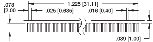
Recommended PCB Layout
