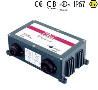
These power supplies have been designed particularly for applications in extreme environments. The rugged die-cast aluminium housing is water, ice, oil and dust resistant in compliance with IP67 and NEMA 4X standards. The metal case works as an efficient heatsink allowing full power operation at up to +60°C ambient temperature (no fan required). With a shock and vibration proof construction the power supplies can be mounted directly on a machine.
