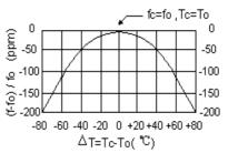
The curve shown above accounts for resonator contribution only and does not include LC component temperature characteristics.
