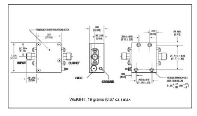
\* Dimensions are inches (millimeters) ±0.015 (0.38) unless otherwise specified.
