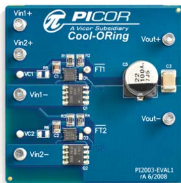
Figure 15: PI2003 Mounted on PI2003-EVAL1
