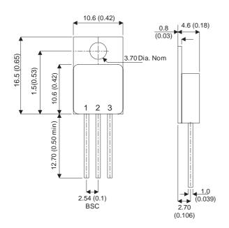
P-Channel MOSFET in a Hermetically sealed TO257AB Metal Package.
