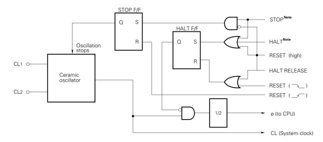
Fig. 2-9 System Clock Generator
