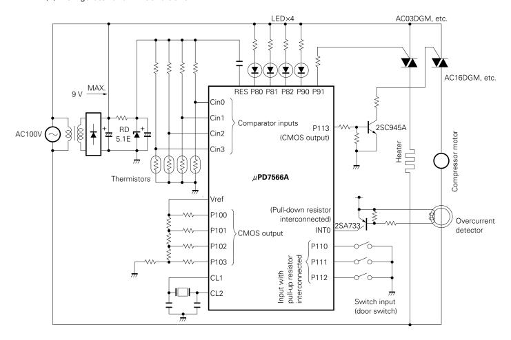
The above example shows a circuit for a refrigerator. A circuit for an air conditioner can be implemented by replacing only the heater with a fan motor.
