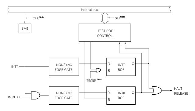
Fig. 2-13 Test Control Circuit
