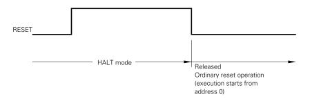
While the RESET signal is active (high level), the HALT mode continues. When the RESET signal goes low, the HALT mode is released. Ordinary resetting operation is then accomplished. Then, the program is executed starting from address 0.
