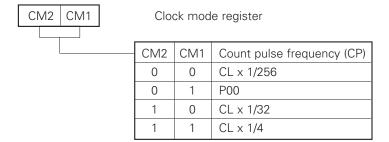
Fig. 2-11 Clock Mode Register Format
