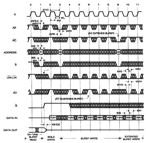
\* When AP is initiates the burst sequence, the W control input is ignored for the first cycle, The W and DATA IN should be asserted and registered in the subsequent cycle.
