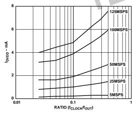
Figure 30. I<sub>DVDD</sub> vs. Ratio @ DVDD = 3 V
