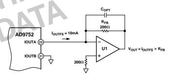
Figure 35. Unipolar Buffered Voltage Output
