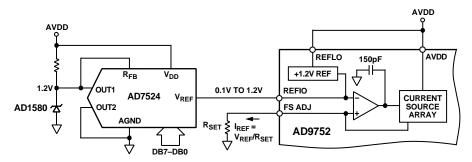
Figure 24. Single-Supply Gain Control Circuit
