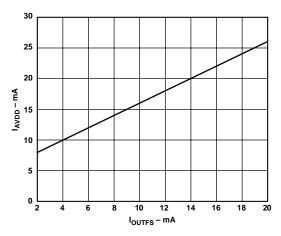
Figure 28. I<sub>AVDD</sub> vs. I<sub>OUTFS</sub>
