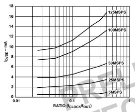
Figure 29. I<sub>DVDD</sub> vs. Ratio @ DVDD = 5 V
