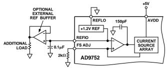
Figure 22. Internal Reference Configuration
