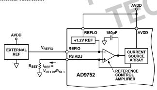
Figure 23. External Reference Configuration
