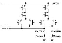
Figure 26. Equivalent Analog Output
