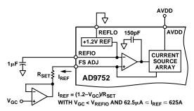
Figure 25. Dual-Supply Gain Control Circuit
