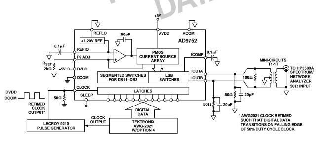
Figure 2. Basic AC Characterization Test Set-Up
