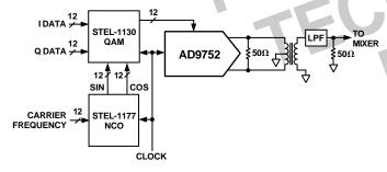
Figure 39. Digital QAM Architecture
