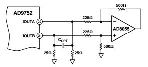
Figure 32. DC Differential Coupling Using an Op Amp
