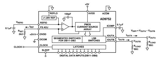
Figure 21. Functional Block Diagram
