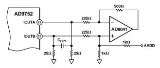
Figure 33. Single-Supply DC Differential Coupled Circuit
