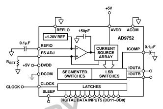
Differential current outputs are provided to support single-ended or differential applications. Matching between the two current outputs ensures enhanced dynamic performance in a differential output configuration. The current outputs may be tied directly to an output resistor to provide two complementary, single-ended voltage outputs or fed directly into a transformer. The output voltage compliance range is 1.25 V.
