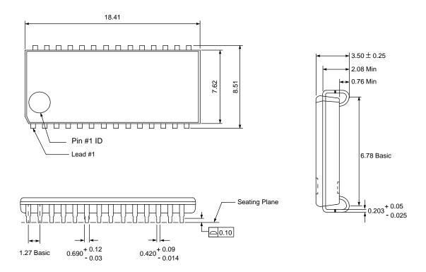
NOTE: All dimensions are in millimeters; Package diagrams are not drawn to scale
