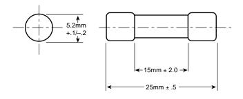
Catalog Symbol: GCF Series Fast-Acting DIN 41576-1 Voltage Rating: 250 Volts AC Interrupting Rating: 300A Opening Times: 1 hour minimum at 150% of rated current 30 minutes maximum at 210% of rated current 300 milliseconds maximum at 400% of rated current 20 milliseconds maximum at 1000% of rated current Physical Size: 5mm × 25mm Construction: Ceramic tube Nickel-plated brass end caps
