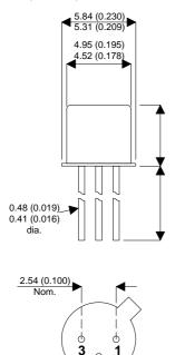
Bipolar PNP Device in a Hermetically sealed TO18 Metal Package.
