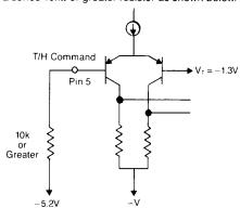
**MN4000 ACQUISITION TIME** — The MN4000's signal acquisition time is specified for full scale steps settling to a specified limit ( $\pm$ 0.1%FSR for 10-bit applications and  $\pm$ 0.01%FSR for 12-bit applications). It is important to note, for the purpose of comparision, that Micro Networks specifies this parameter from the edge of the
