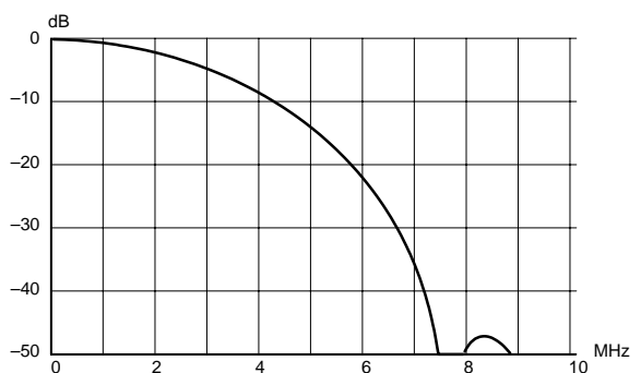
Fig. 2–6: Frequency response of the chroma interpolation filter
