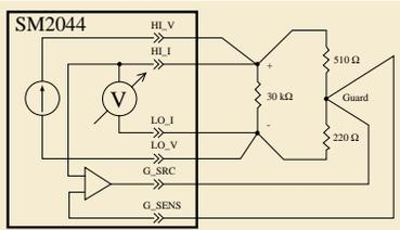
Example: Assume a 30kΩ resistor is in parallel with two resistors (510 Ω and 220 Ω), that are connected in series. By sensing the voltage at the top of the 30 kΩ, and then applying this same voltage to the junction of the 510 Ω and 220 Ω there is no current flow through the shunting path. With this "guarding", the SM2044 accurately measures the 30kΩ resistor.
