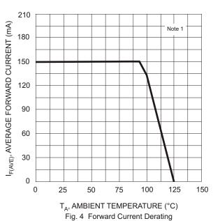
Note 1: Part mounted on FR-4 board with recommended pad layout, which can be found on our website at http://www.diodes.com/datasheets/ap02001.pdf.
