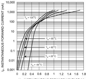
V<sub>F</sub>, INSTANTANEOUS FORWARD VOLTAGE (V) Fig. 1 Typical Forward Characteristics
