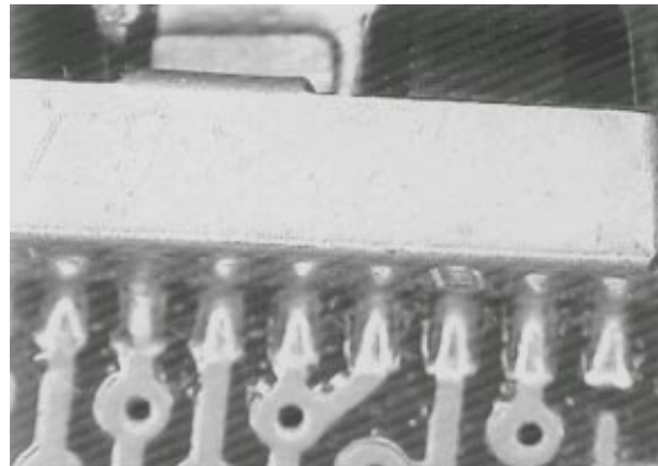
Photo 4.0. Unit self-aligns after reflow.
