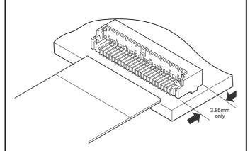
Space saving flip lock type connector, with 1.8mm height and 3.85mm depth.
