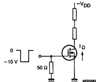
Fig.3 Switching times test circuit.
