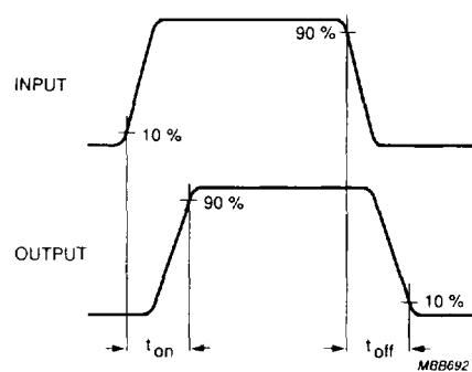
Fig.4 Input and output waveforms.
