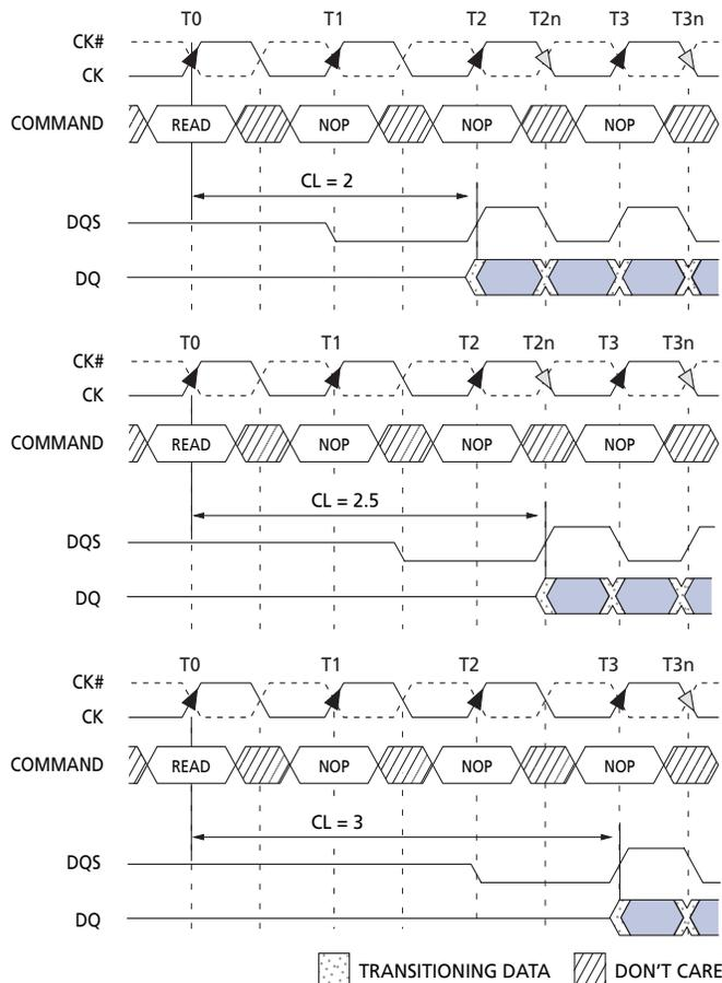
Note: Burst Length = 4 in the cases shown; shown with nominal  $t_{AC}$ ,  $t_{DQSK}$ , and  $t_{DQSQ}$ .
