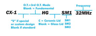
**Total Frequency Tolerance** 50ppm **25ppm** Calibration **Temperature Frequency Tolerance\* Stability** Range: @ 25°C over **C** = **C**ommercial A, B, C **Temperature** I = Industrial Range M = Military S = Specify \*For other calibration tolerances enter figure in ppm
