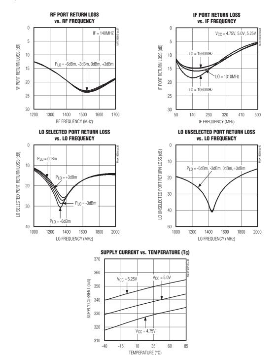
(*Typical Operating Characteristics (continued*) (*Typical Application Circuit* (see Table 1). Vcc = 3.3V, f<sub>RF</sub> > f<sub>LO</sub> for a 140MHz IF, P<sub>RF</sub> = -5dBm, P<sub>LO</sub> = 0dBm, T<sub>C</sub> = +25°C, unless otherwise noted.)
