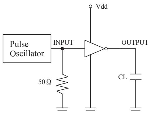
\* Output should be opened when measuring current consumption.
