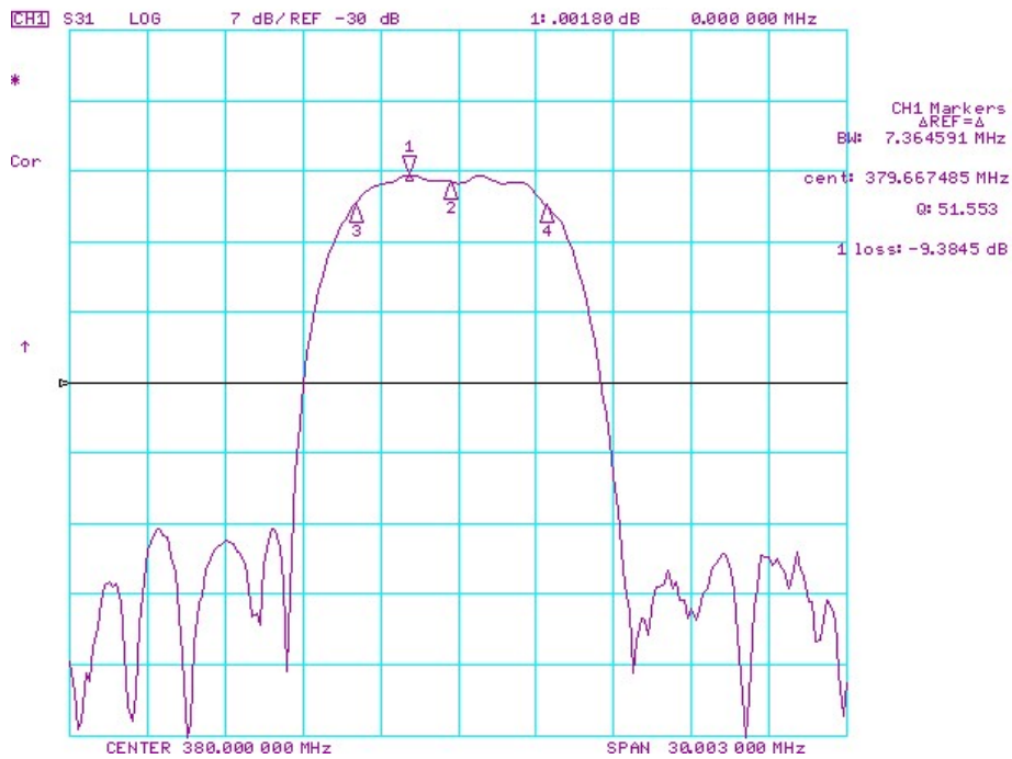
Fig-1 S21 Response Horizontal: 3MHz/Div Vertical: 7dB/Div
