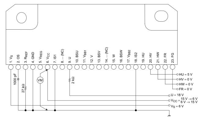
\*: Sweeps the V<sub>CC</sub> pin voltage from 15 V to decrease and monitors the U pin voltage.
