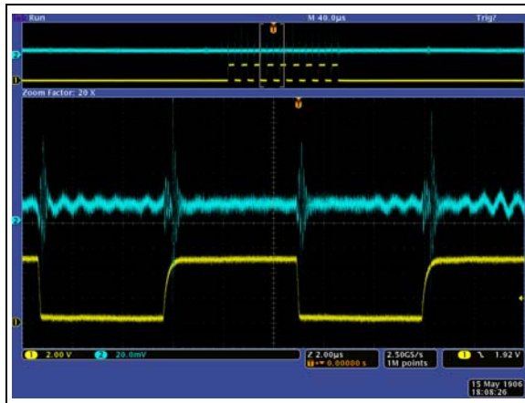
FIGURE 2-40: Digital Feedthrough (SCL signal coupling to V_{OUT} pin); V_{DD} = 5.0\text{V} , V_{REF} = 5.0\text{V} , F_{SCL} = 100\text{ kHz} , V_{OUT} = 20h ( V_{OUT} Voltage Scale = 20\text{ mV/div} , Time scale = 2\ \mu\text{s} / \text{div} ).
