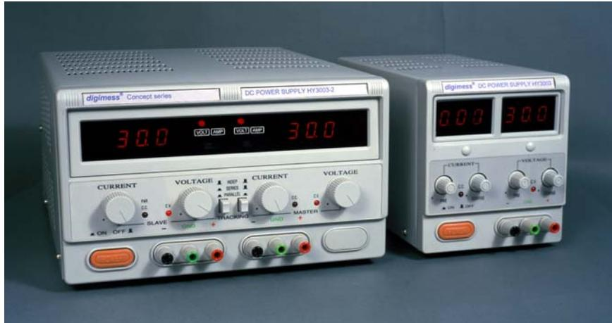
The *digimess*<sup>®</sup> HY series is a comprehensive range of low cost general purpose linear power supply units containing single, dual and triple output models. All models can operate in either constant voltage or constant current modes and feature large red LED displays for ease of viewing.
