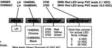
\*Wire leads 24awg Stranded UL1007 80C Black and Red 5" min length 1/4" strip. Consult factory for alternative lengths.
