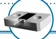
The PCS-P series split ground high power thin film terminator combines the improved heat dissipation of a double-sided flange and the split ground to give a power rating of up to 80W, while providing excellent high frequency characteristics from DC to 1.5 GHz. Attaching the flange directly to a heat sink provides improved heat dissipation at a higher power rating. Typical applications include aerospace, wireless communication, satellites and RF power amplifiers.
