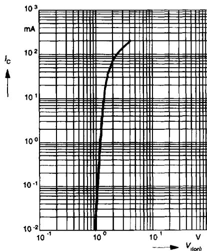
**Collector-Emitter Saturation Voltage**
