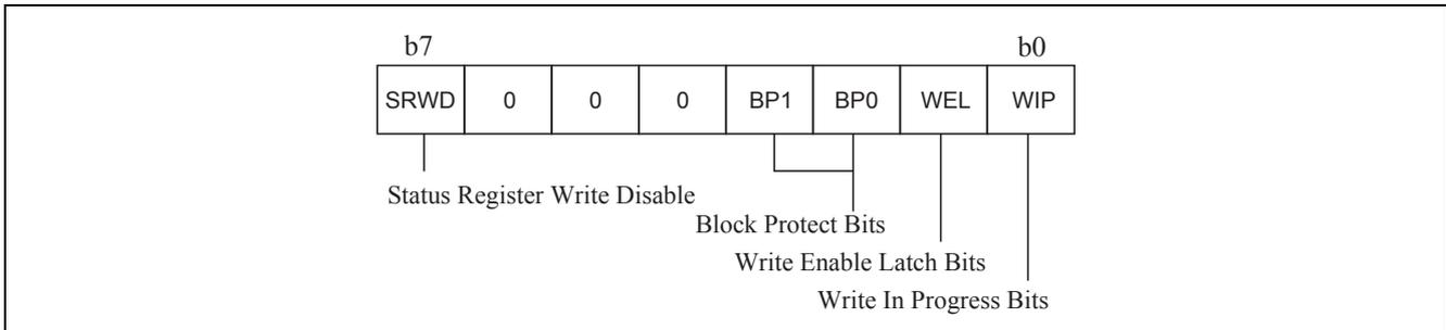
**WIP bit:** The Write In Progress (WIP) bit indicates whether the memory is busy with a Write or Write Status Register cycle.
